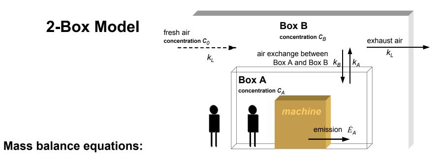
$V_{A}$  = volume box A  $V_B$  = volume box B t = working time 8h  $\dot{E}_{A}$  = emission rate into box A
